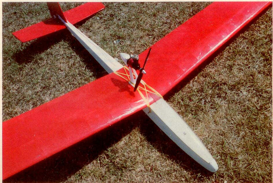
A power pod may be used - this is the Cox unit with a Texaco .049 in place.
