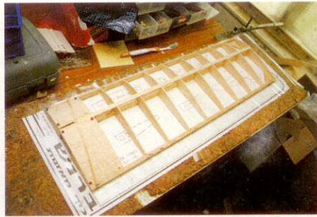
ABOVE LEFT: The fuselage top sheet is rebated for a strong and perfect joint. ABOVE CENTRE: Everything fits, even the sheet is cut to size and marked 'top' or 'bottom'. ABOVE RIGHT: Simple, strong wing is easy to build and easy to repair.
